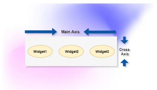
The column's cross-axis will run horizontally and the main axis will run vertically. The following figure will clarify the concept more.
